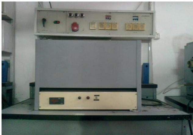
Figure 2.3 – SUOL-044 12-M2 tubular electric furnace
