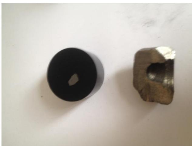
Figure 4.4 - Smelted metal samples (second stage of metallization with dissolved carbon)
