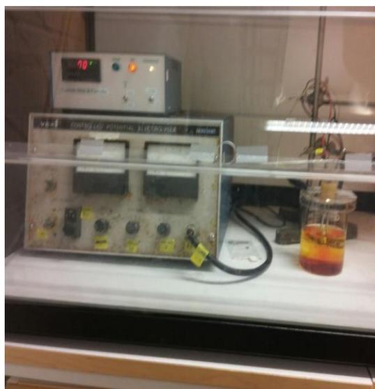
Figure 2.6 - Device for the detection of non-metallic impurities by electrolytic extraction
