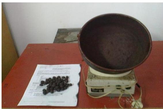
Figure 2.2 – Disc granulator
